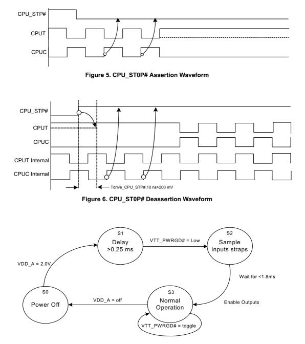
Figure 7. Clock Generator Power-up/Run State Diagram
