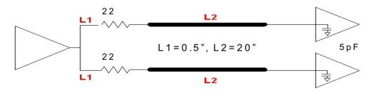
Figure 9. Single-ended REF Load Configuration
