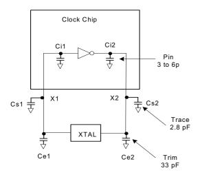
Figure 2. Crystal Loading Example
