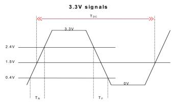
Figure 10. Single-ended Output Signals (for AC Parameters Measurement)
